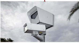
The SensorTec Speed Detection Radar Camera system is used to detect multiple over speeding vehicles using the radar module, then sends the metadata to camera's VCA software which recognizes the over speeding vehicles and their number plates and sends it to violation management server.
